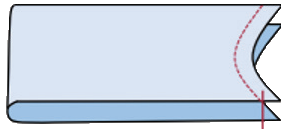
Rib collar folding and sewing with single lockstitch stitches
